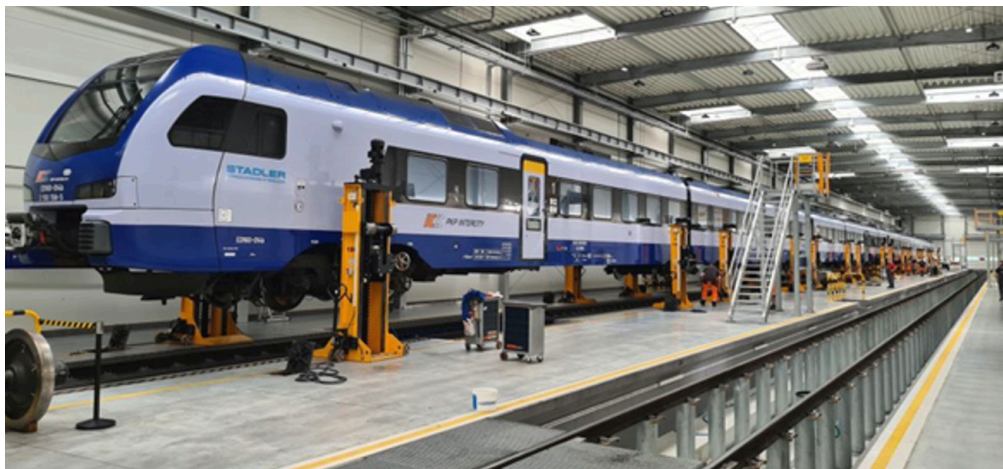
FIGURE 32: EMU RAISED ON SYNCHRONIZED JACKS *Photo Courtesy of Stadler
