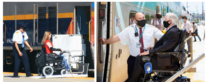
FIGURE 24: BOARDING LIFT MECHANISM FULLY DEPLOYED
