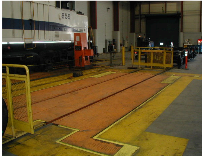
FIGURE 30: CMF LOCOMOTIVE SHOP, WITH DROP TABLE
