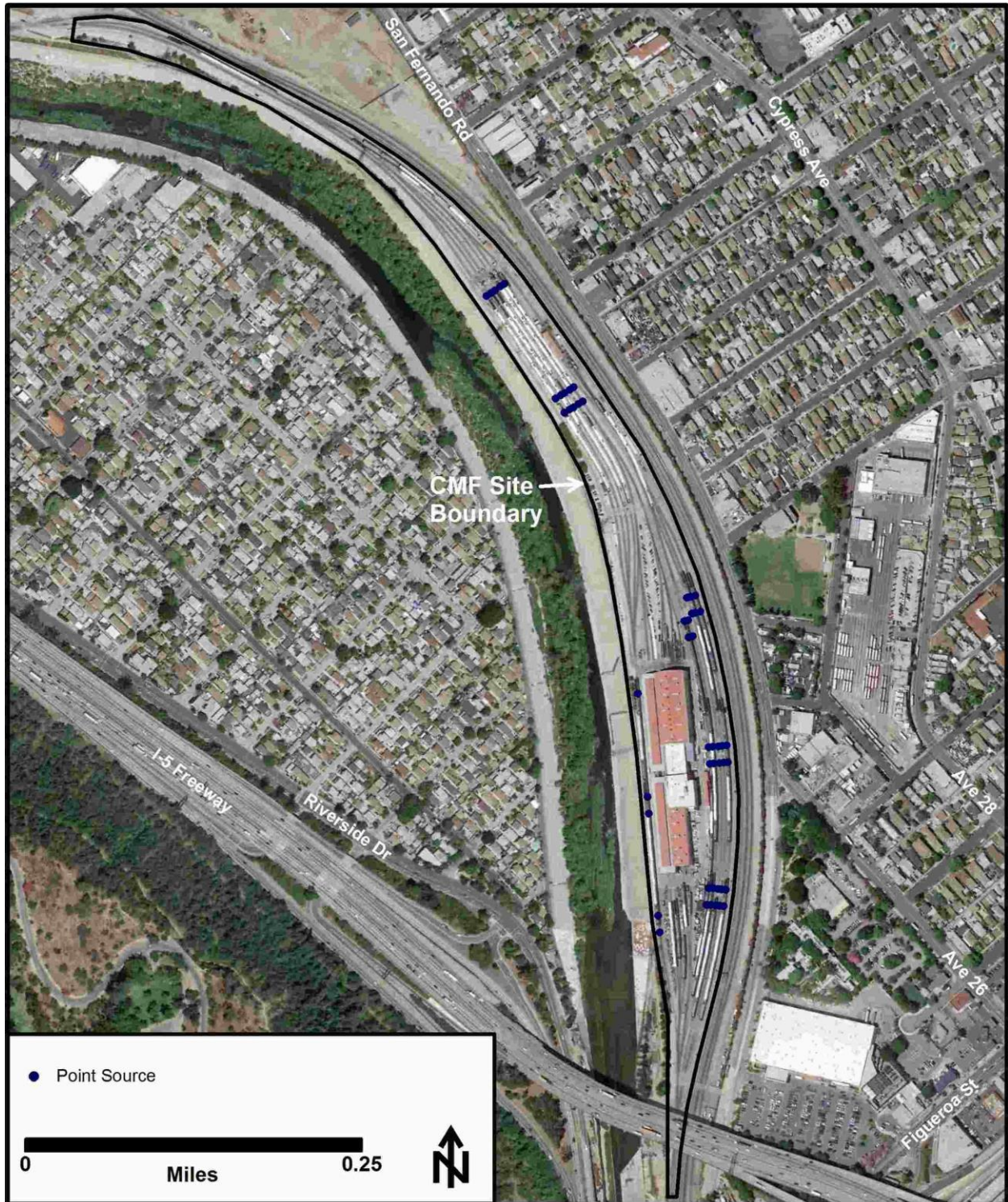
Figure D-7. AERMOD Source Representation – HEP Engines on Stationary Trains at the CMF – All Years
