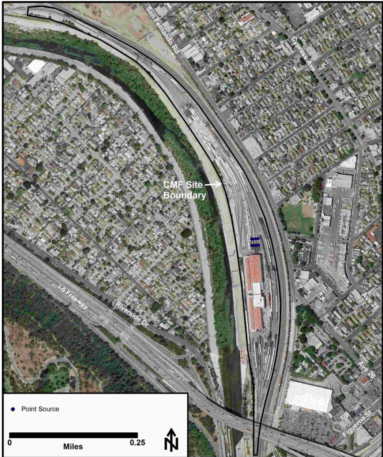
Figure D-4. AERMOD Source Representation – Locomotive Load Testing at the CMF – All Years
