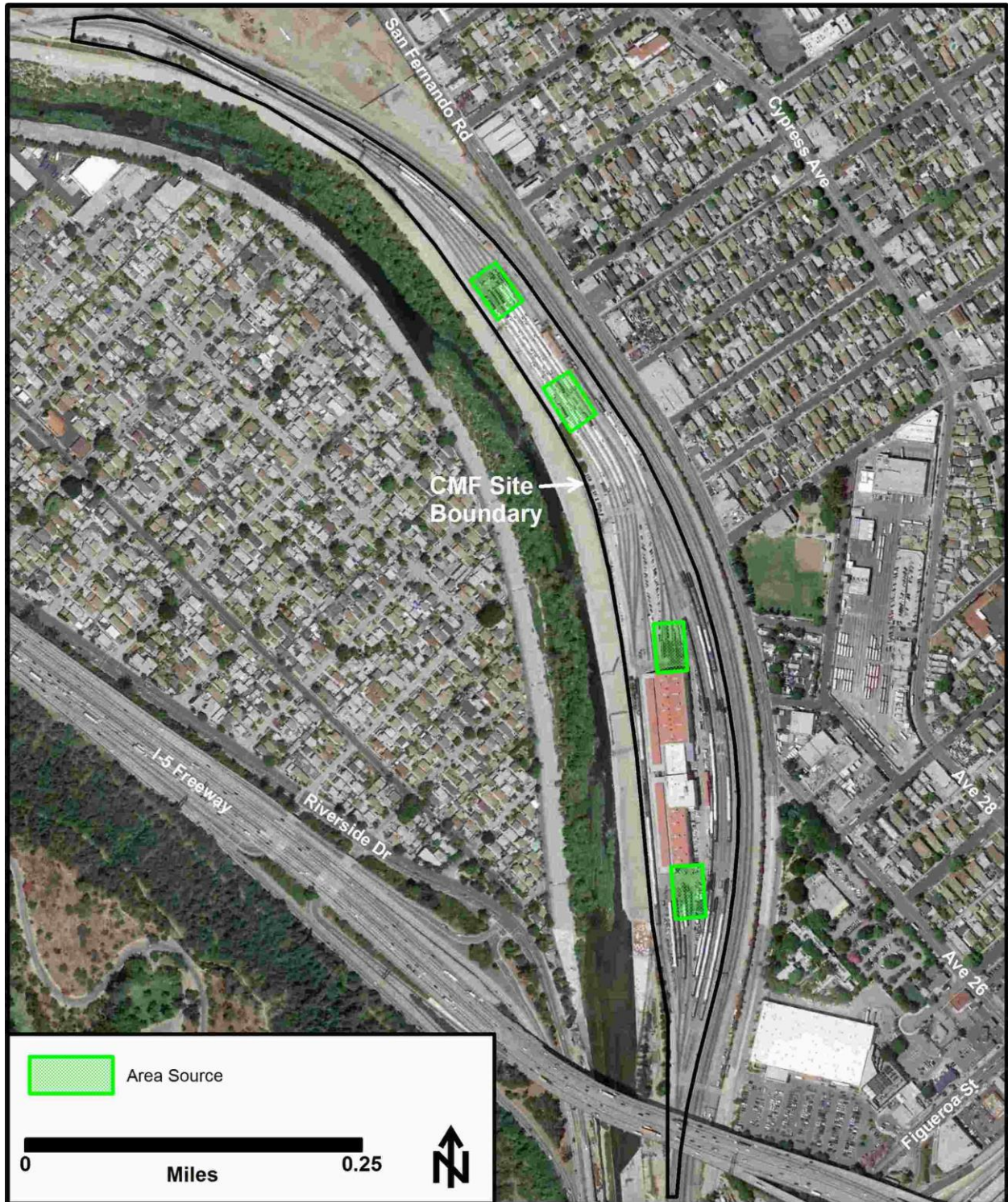
Figure D-12. AERMOD Source Representation – Diesel Forklifts and Welder at the CMF – All Years
