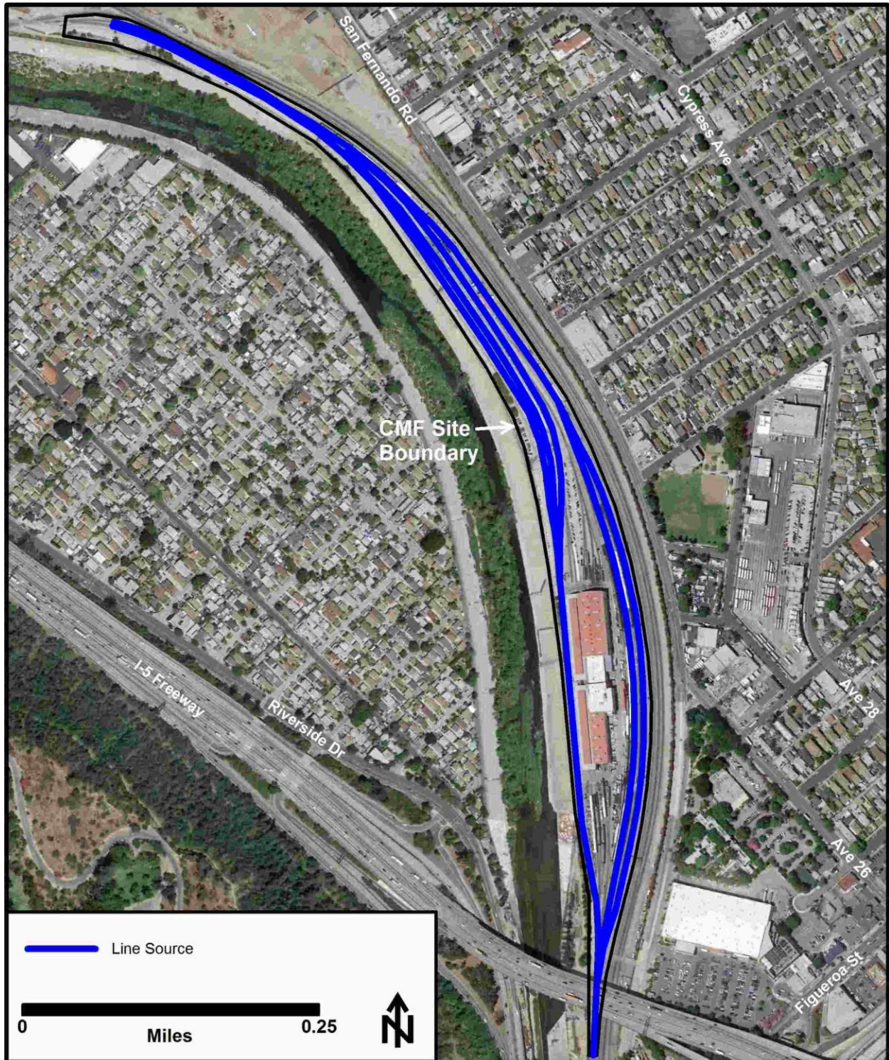
Figure D-5. AERMOD Source Representation – Locomotives on Moving Trains at the CMF – All Years
