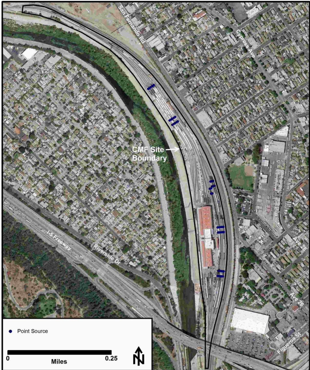
Figure D-3. AERMOD Source Representation – Locomotive Brake Testing at the CMF – 2012, 2014, and 2017
