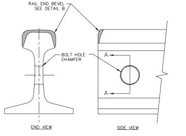
RAIL CHAMFERING AND BEVELING
