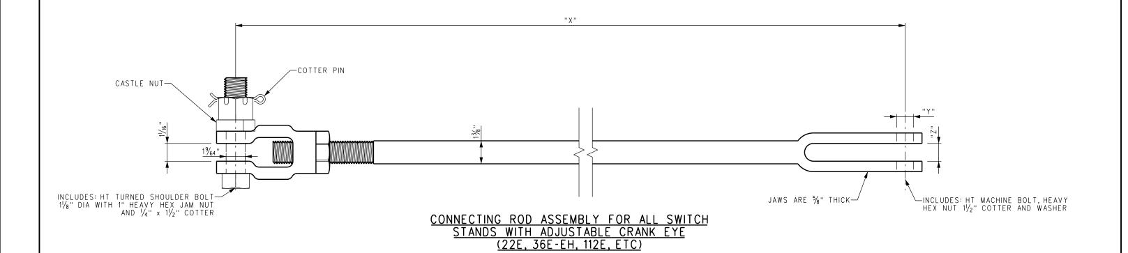
"Y" -  $1\frac{1}{64}$ " FOR  $\frac{3}{4}$ " AND 1" HEAD RODS - 1%4" FOR 11/4" HEAD RODS
