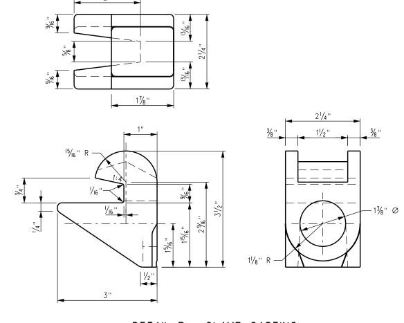
DETAIL B - CLAMP CASTING
