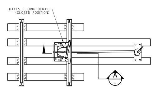
GENERAL PLAN FOR CONNECTING ROD WITH HAYES SLIDING DERAIL
