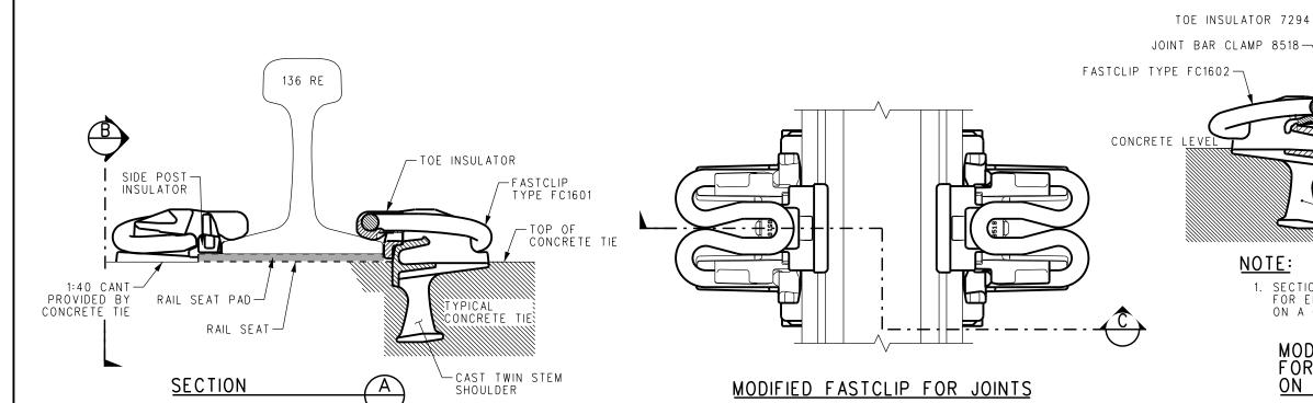
NOTE: SECTION C PROVIDES A VIEW OF A MODIFIED FASTCLIP FOR EITHER A STANDARD JOINT OR AN INSULATED JOINT ON A CONCRETE TIE.
