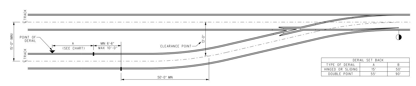
TURNOUT - DERAIL NOT CONNECTED TO SIGNAL SYSTEM - OUTSIDE INSULATED JOINTS
