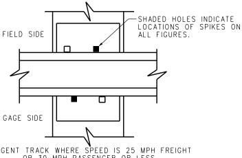
TANGENT TRACK WHERE SPEED IS 25 MPH FREIGHT OR 30 MPH PASSENGER OR LESS YARD AND INDUSTRY TRACK < 6° CURVES
