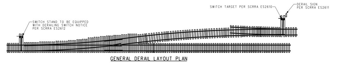
SEE SCRRA ES2702 FOR DISTANCE FROM MAIN TRACK SWITCH TO POINT OF DERAIL AND INSULATED JOINT LOCATIONS.
