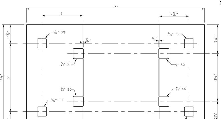
1. ALL SQUARE SPIKE HOLES SHALL HAVE 1/6" FILLETS IN CORNERS. 2. ESTIMATED WEIGHT: 19.60 LBS EACH. 3. MUST MEET AREMA SPECIFICATIONS.
