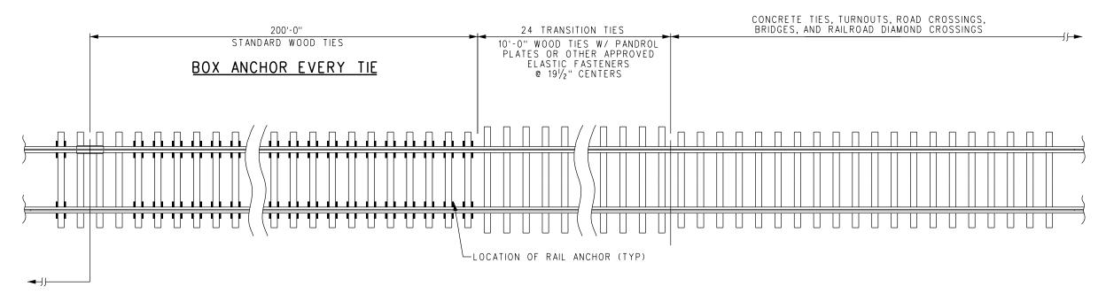
STANDARD RAIL ANCHOR PATTERN PER SCRRA ES2351-02 IF CWR, AND SCRRA ES2351-01 IF JOINTED RAIL
