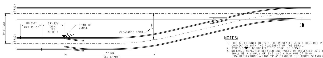
TURNOUT - DERAIL CONNECTED TO SIGNAL SYSTEM
