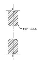
**BOLT HOLE CHAMFER** SECTION A-A
