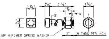
**BOLT FOR REPLACING LOOSE RIVETS**
