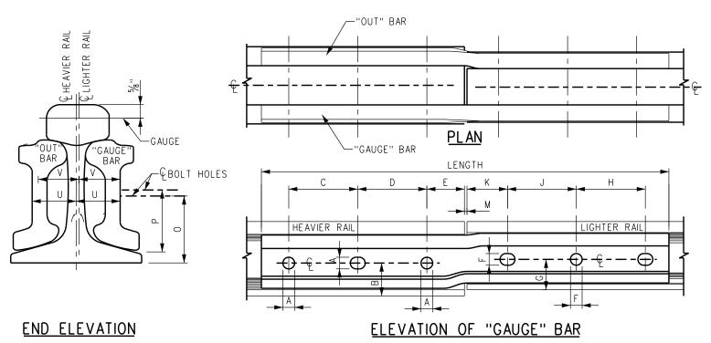
2. USE STANDARD JOINT BAR PER ES2501, MACHINED & LABELED TO INDICATE RAIL SIZE AND GAUGE AND FIELD SIDES.
