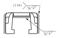
TYPICAL SAFELOK WELD-ON CAST SHOULDER WELDING DETAILS
