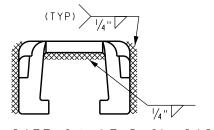
TYPICAL SAFELOK WELD-ON CAST SHOULDER WELDING DETAILS
