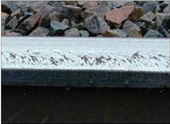
Severe Flaking with Head Checking
