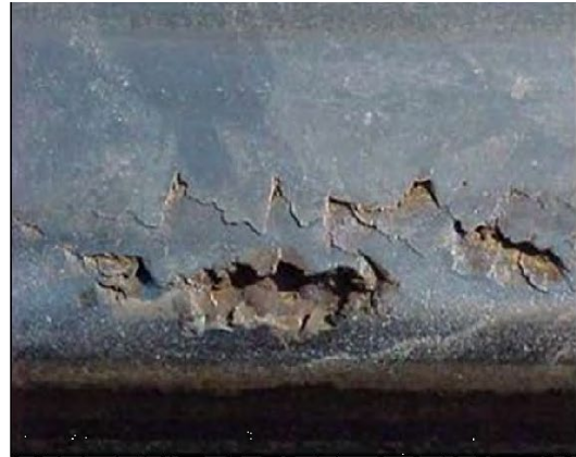
Close Up of Flaking on Gage
