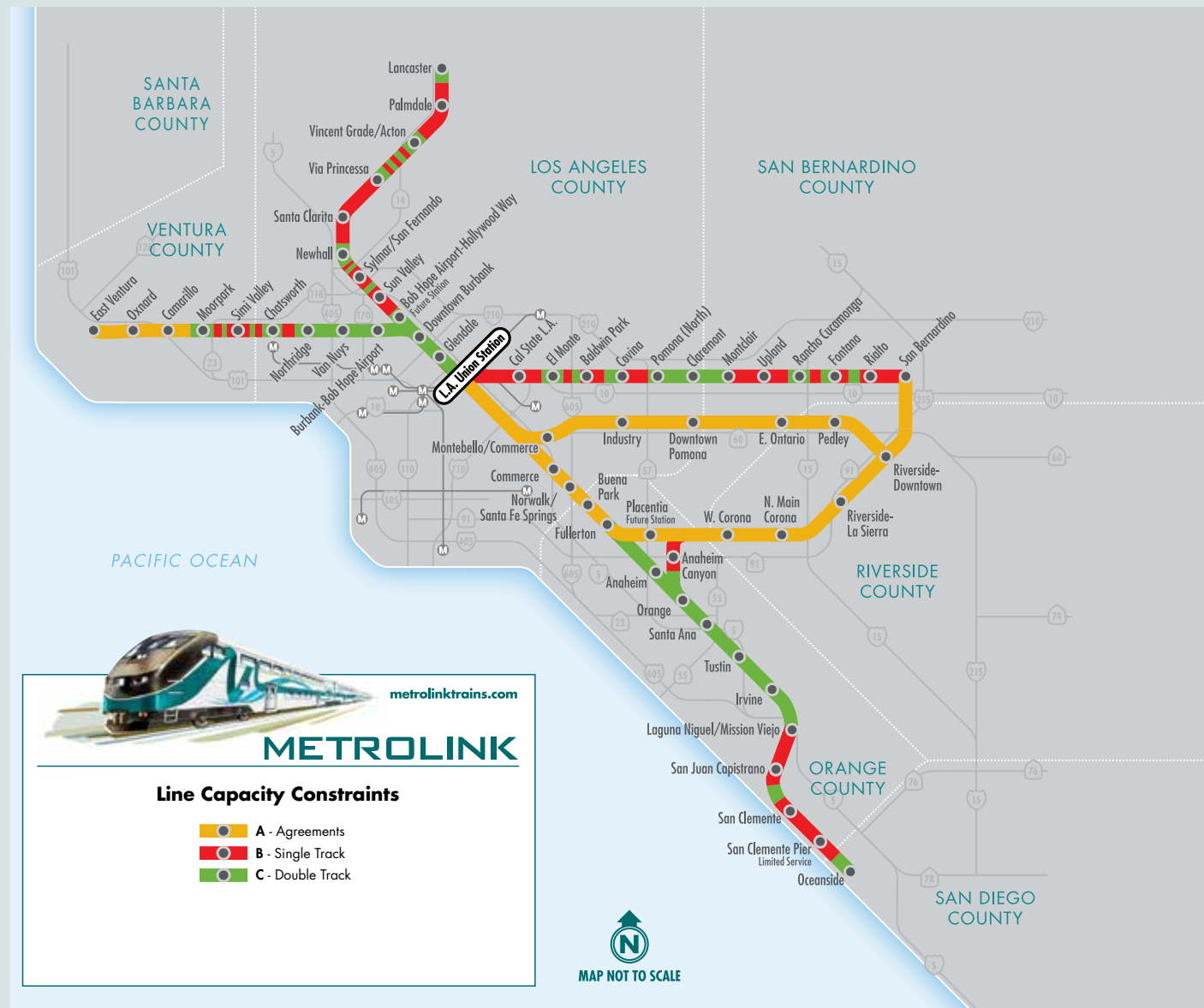
Figure 10: Existing Metrolink Network Line Capacity Constraints
