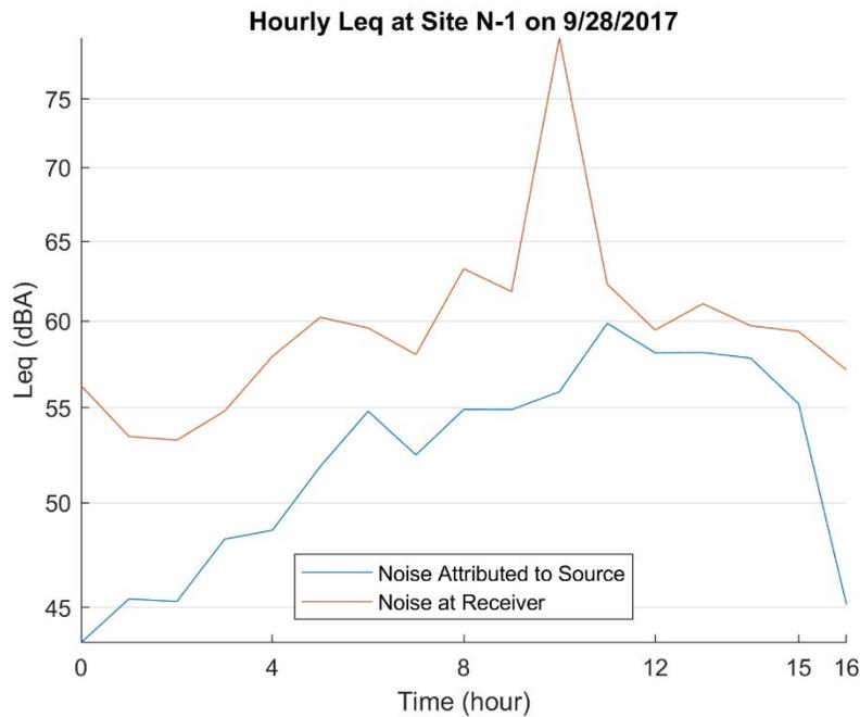
**Figure 5: The hourly noise levels at N-1 for 9/28/17. The orange line is the raw measured data while the blue represents the noise levels attributed to the CMF.**
