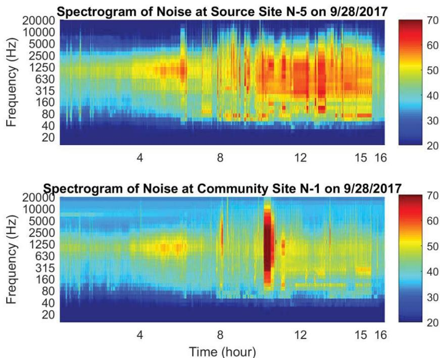
**Figure 2: Spectrograms of measured noise at two monitoring sites for 9/28/17**
