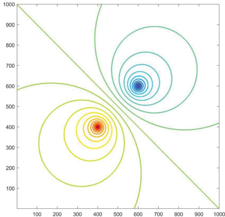
**Figure 6: Contour plot of lines of equal noise difference between two monitoring locations**
