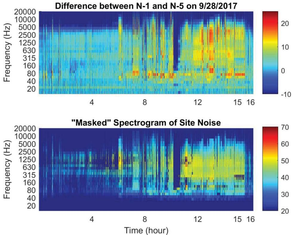
**Figure 4: The top plot shows the difference spectrogram calculate from those of N-1 and N-5. The lower plot shows the masked spectrogram of noise at N-1 after extraneous events have been removed.**
