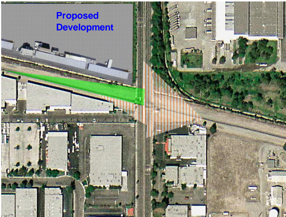
Figure 3-17. Sight Triangle Impeded by Adjacent Buildings
