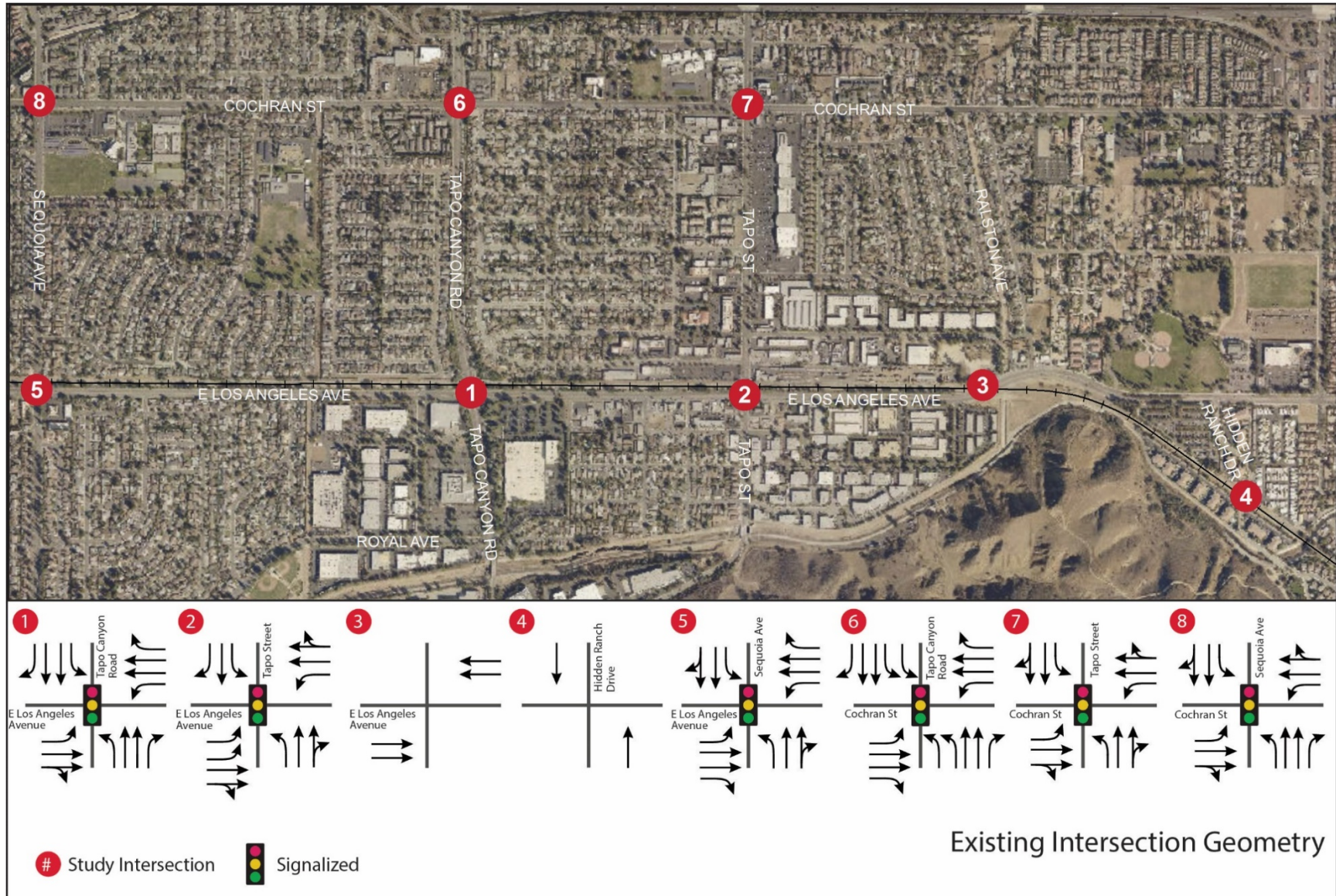
Figure 4-2. Existing Intersection Lane Configuration
