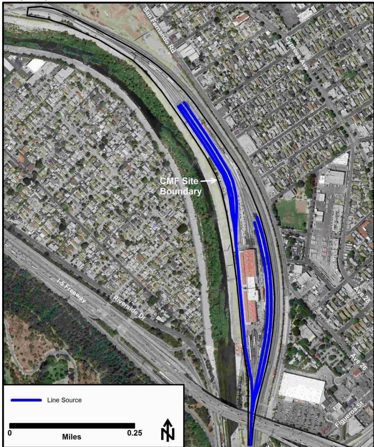
Figure D-10. AERMOD Source Representation – HEP Engines on Moving Trains at the CMF – 2012, 2014, and 2017
