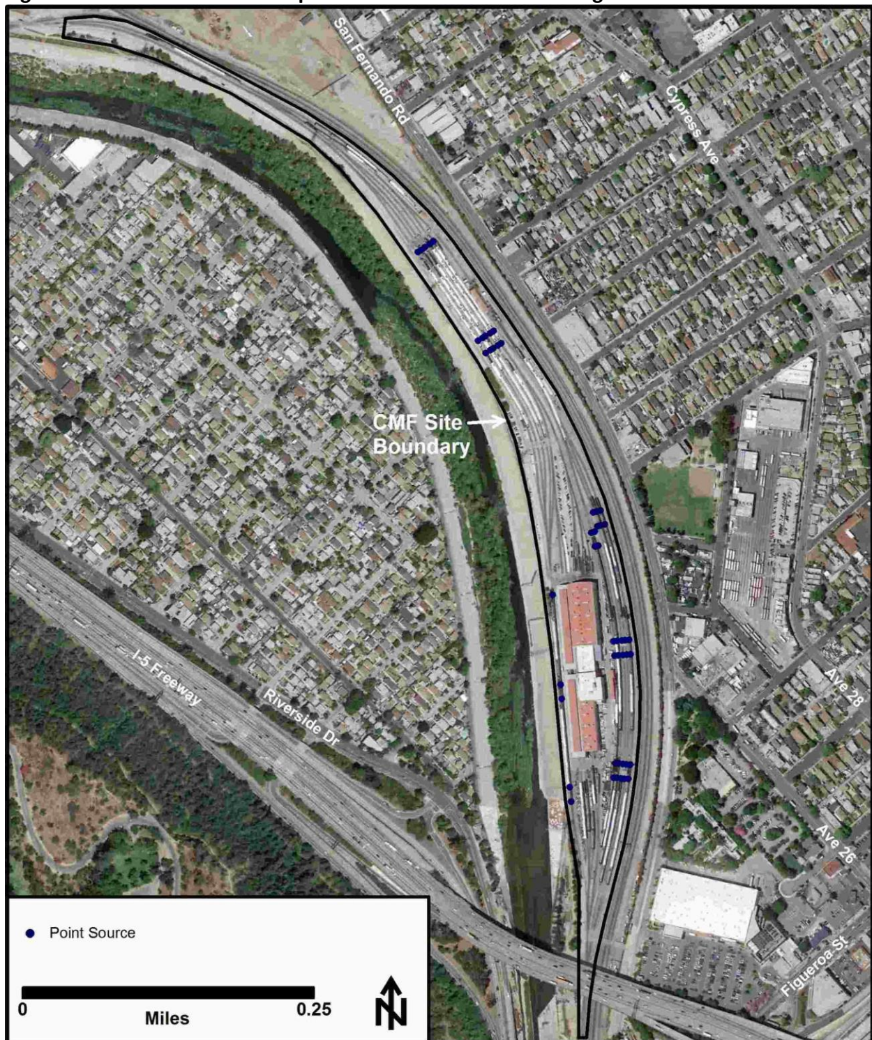
Figure D-1. AERMOD Source Representation – Locomotive Idling at the CMF – All Years
