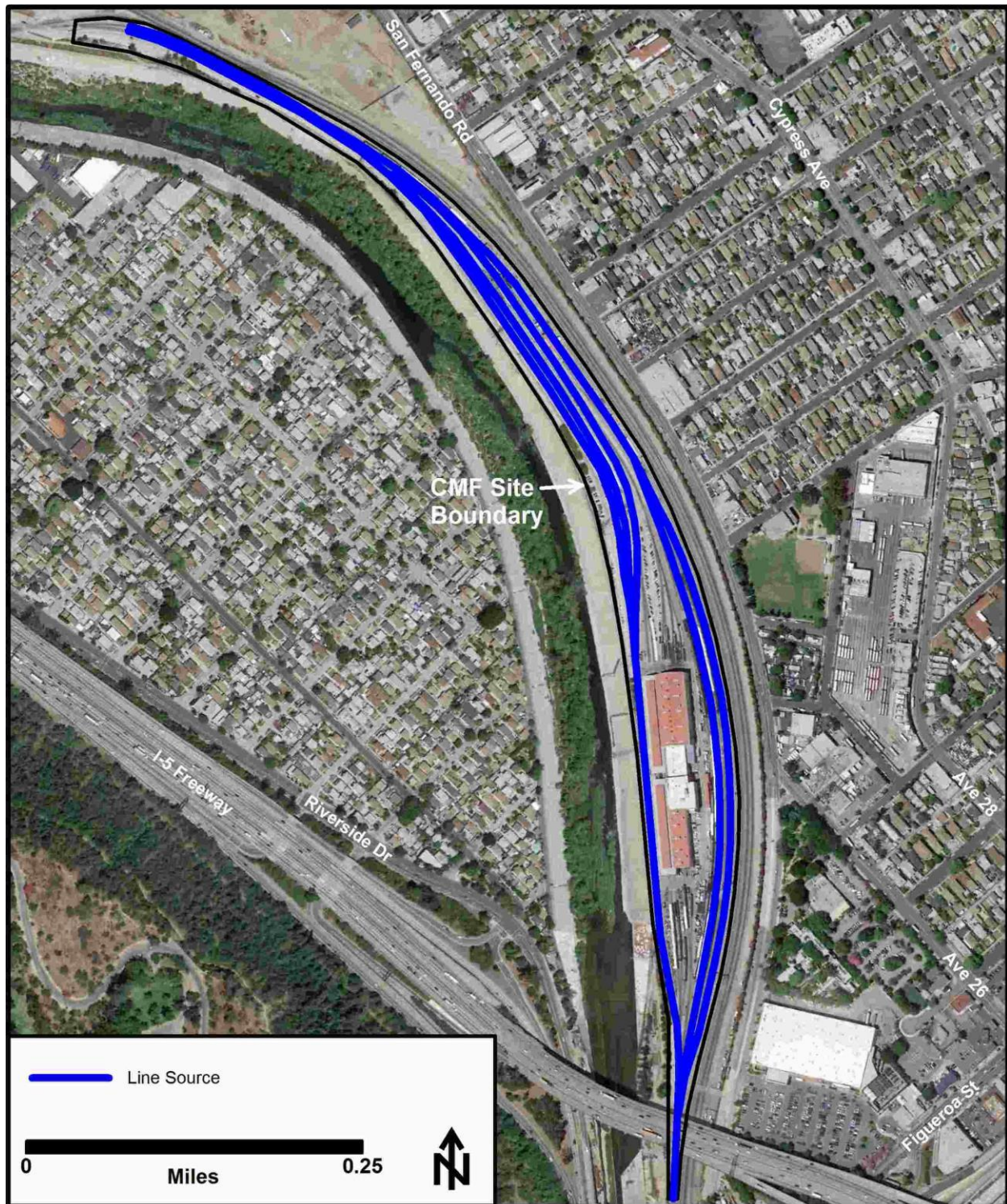
Figure D-9. AERMOD Source Representation – HEP Engines on Moving Trains at the CMF – 2010
