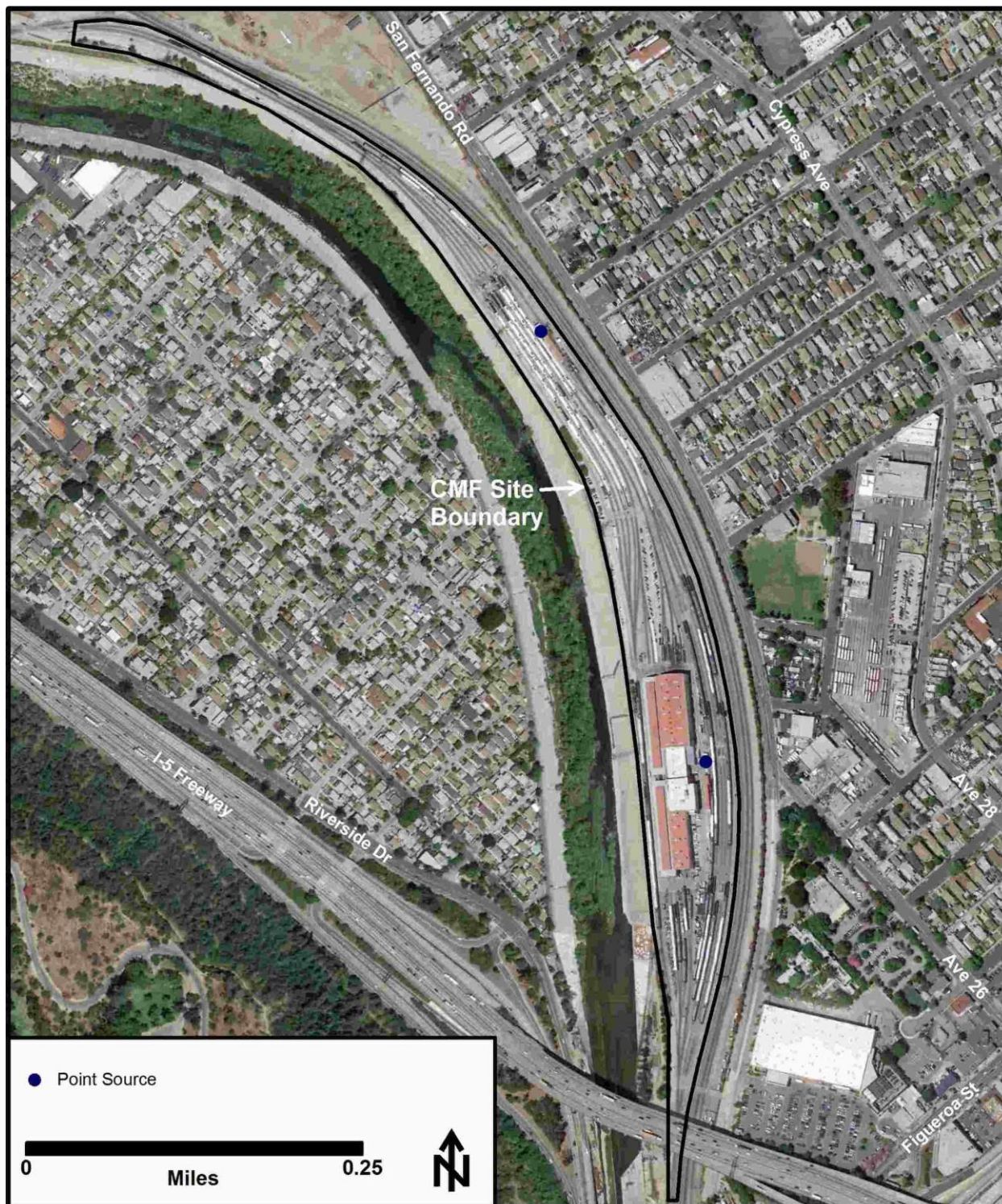
Figure D-11. AERMOD Source Representation – Standby Diesel Generators at the CMF – All Years
